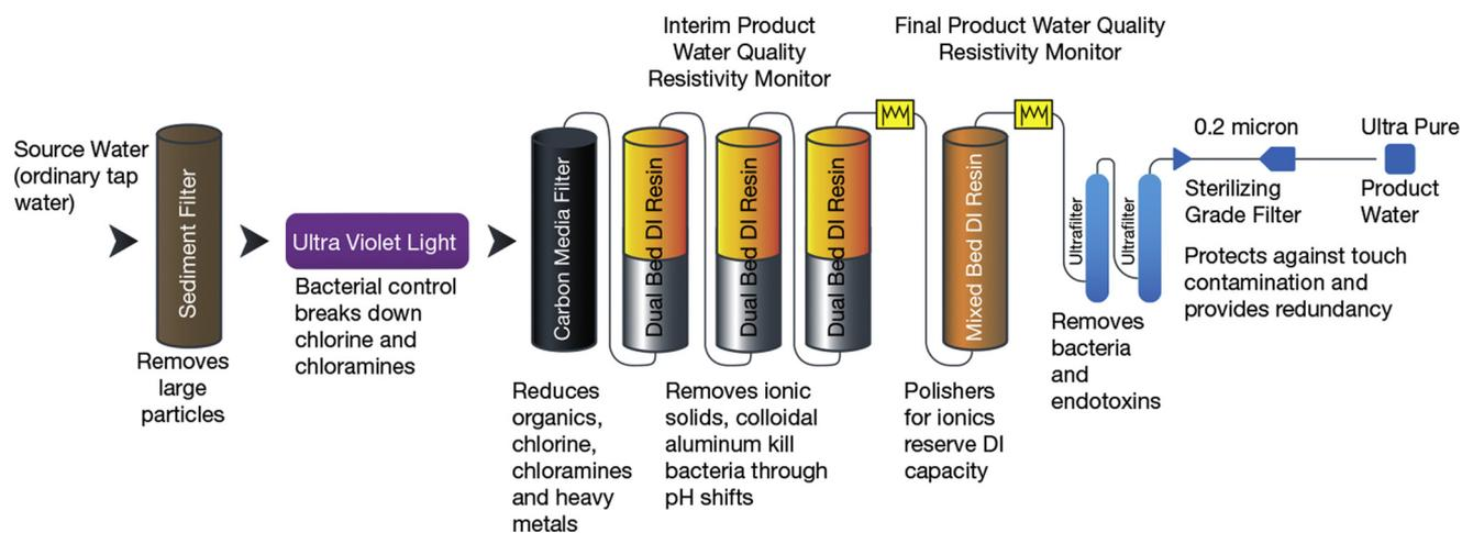
**Figure 1.** NxStage PureFlow Purification Pack water purification system. Image ©2019 NxStage Medical, Inc; reproduced from *Therapy Handbook: NxStage Hemodialysis Treatment* with permission of the copyright holder.
